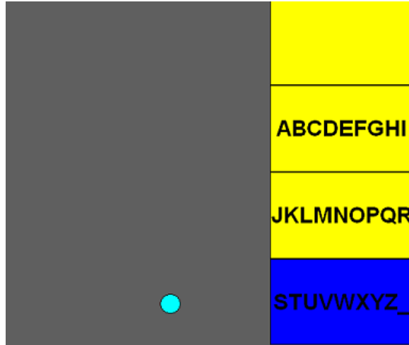
Figure 2.2: The Thought Translation Device [29]. The left to right movement of the cursor is constant; the vertical movement is controlled by the user’s brain activity. A letter is selected by sequential selection of blocks of letters presented in a dichotomic structure.
