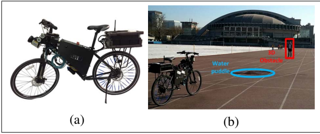
Fig. 9. (a) The implemented autonomous bicycle and (b) our experimental venue for obstacle detection and avoidance.
